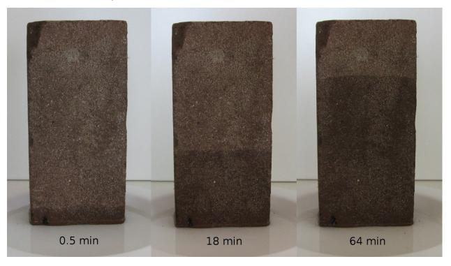
Capillary water flow in a brick that is in contact with water at the bottom. The time elapsed after first contact with water is indicated. The brick height is 225 mm (about 9 inches). From the weight increase, the estimated porosity is 25%. Think about how tall a redwood tree is: that's how high water can climb in wood. Photo: Hankwang via wikicommons
